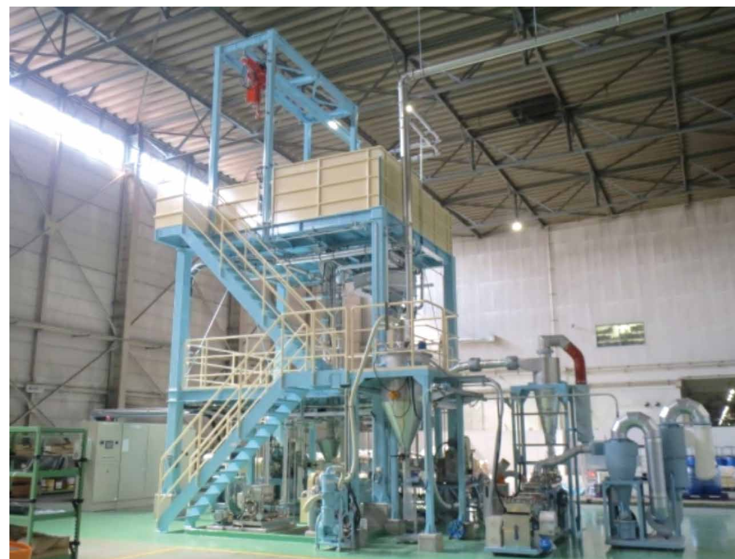
CNF強化樹脂実証生産設備 Pilot production equipment of CNF-reinforced plastics
