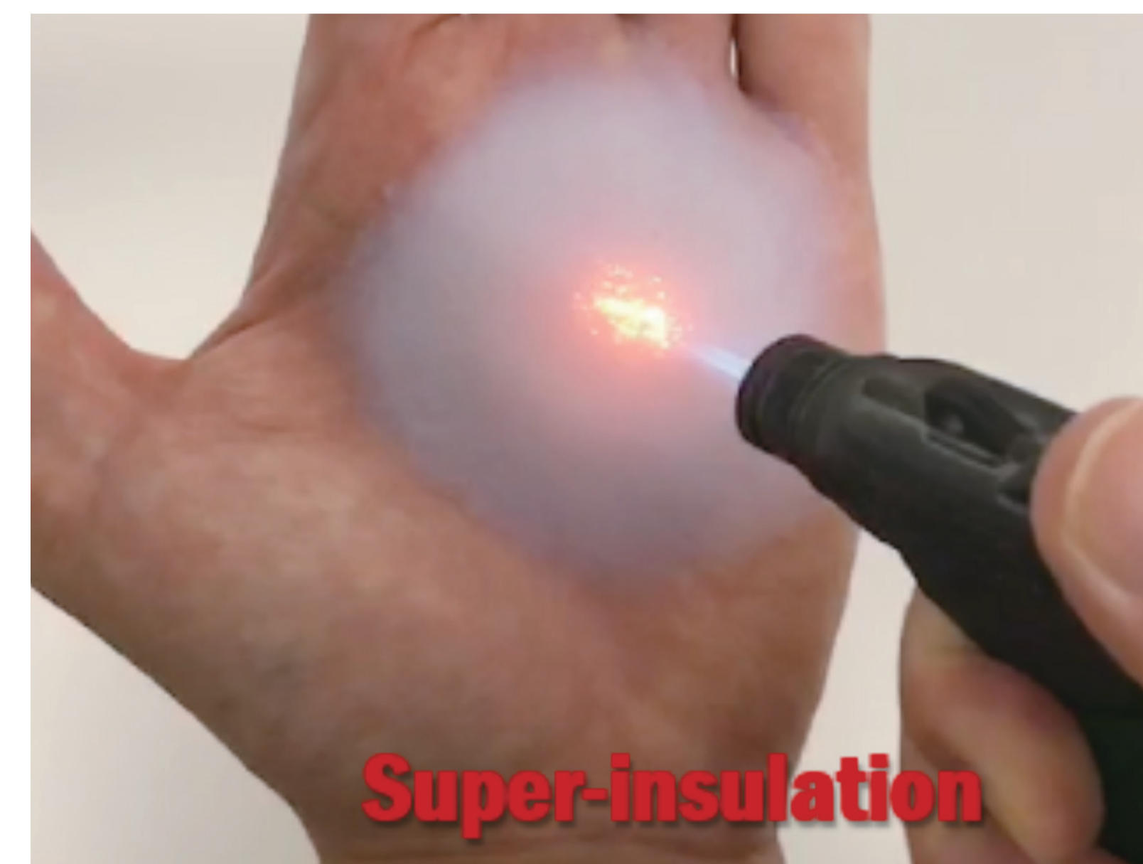
3mm厚に盛ったTIISA®が1300℃の炎を防ぐ The 3mm TIISA® is guarding against a 1300°C flame
