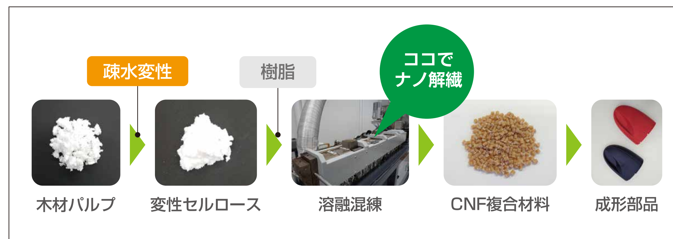
Fig. 1 CNF/Resin Composite Manufacturing Process
