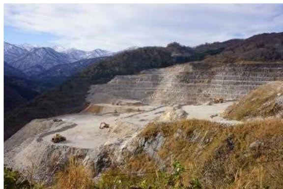
Extraction of **limestone (CaCO<sub>3</sub>)** to produce cement, etc.
