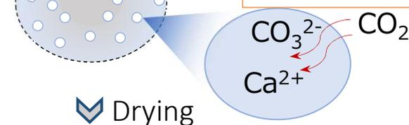
Rapid precipitation in pores
