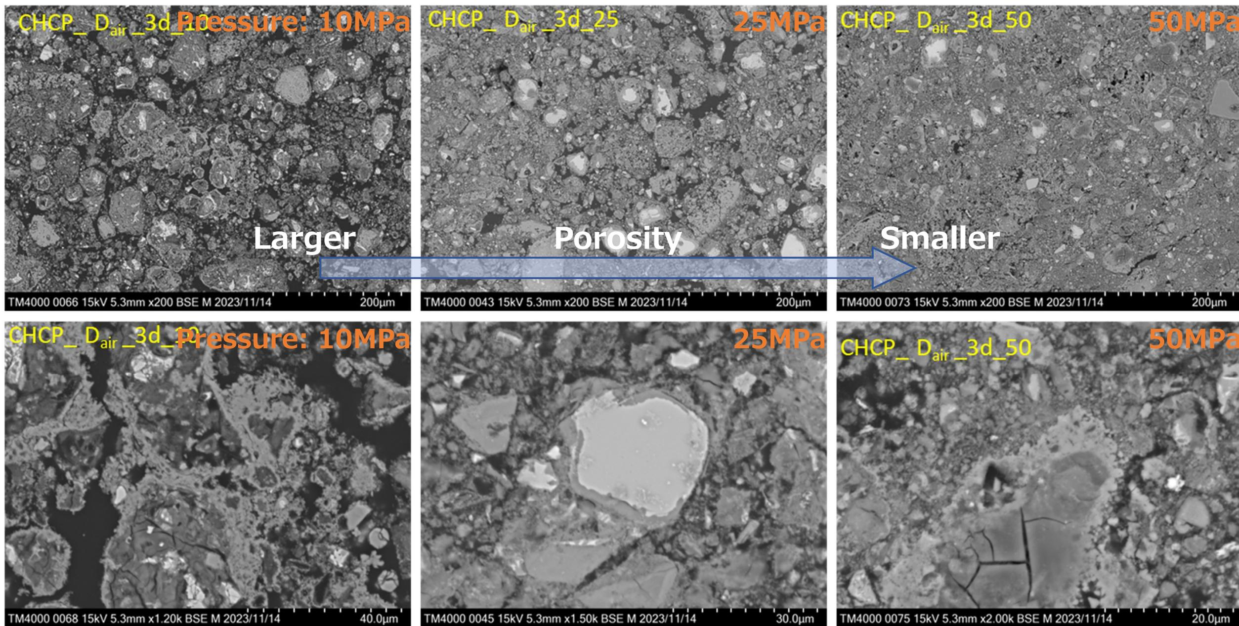
■ Increasing pressure decreases porosity and increases compressive strength of CCC.
