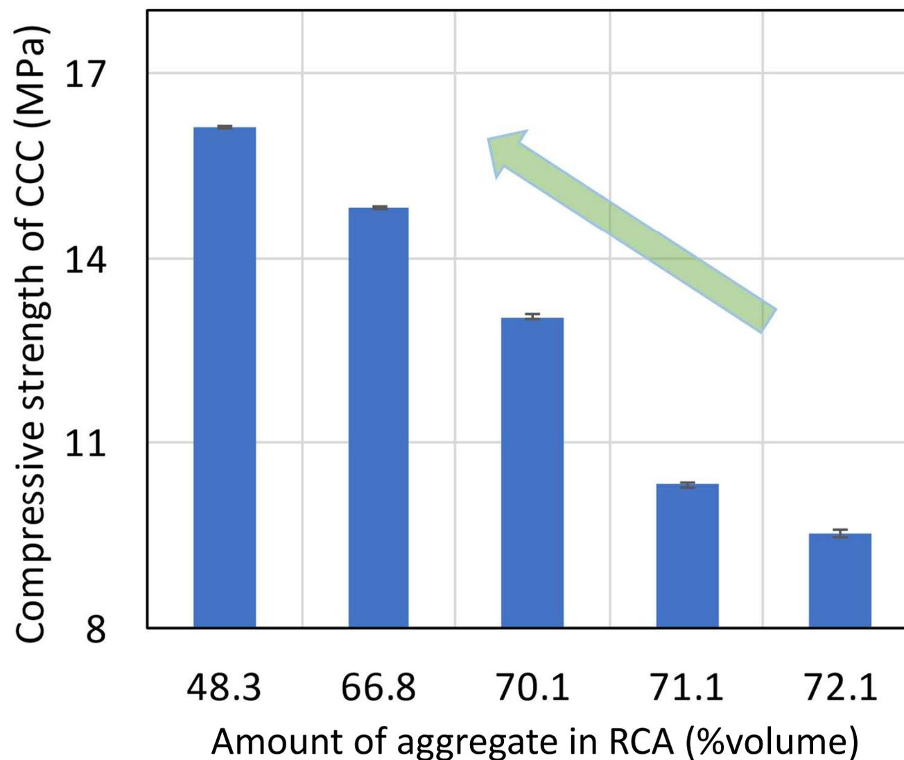
■ The lower the amount of aggregate in the waste concrete
