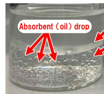
absorbent(oil) phase & aqueous phase liquid-liquid separation
