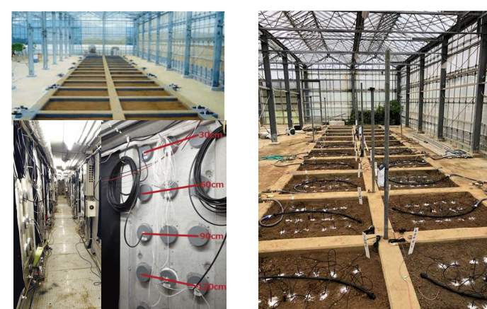
Fig. 04-2. In-house lysimeter experiment to quantify carbon budget changes caused by ERW application@Ishigaki
