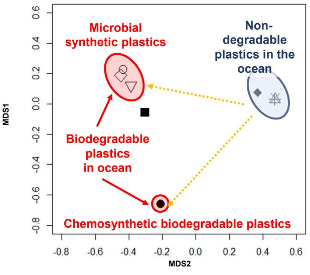
Addition of 10% plastisphere control substance candidate to the biodegradable base polymer. The films were exposed to seawater and investigated weight loss and change in plastisphere.
