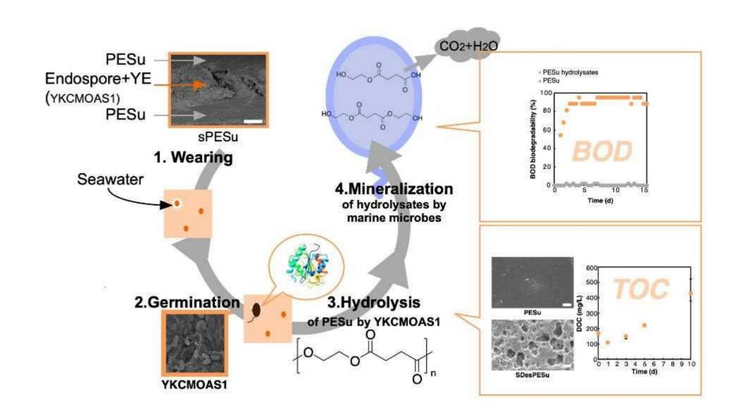
PESu degraded in the marine environment by spore-forming bacteria was eventually mineralized in the marine environment.
