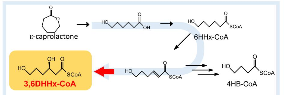
Develop PHA polymerases that efficiently polymerizes 3,6DHHx-CoA produced from  $\epsilon$  caprolactone by metabolism
