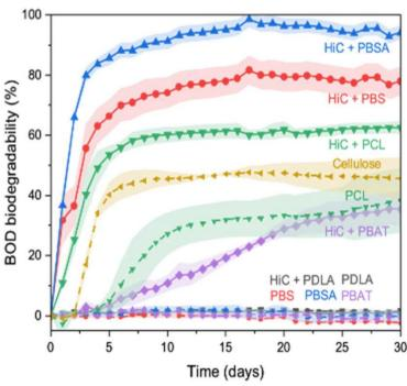
Normal biodegradable plastics hardly degrade in seawater, but enzymatic encapsulation proved to be more degradable than cellúlose.
