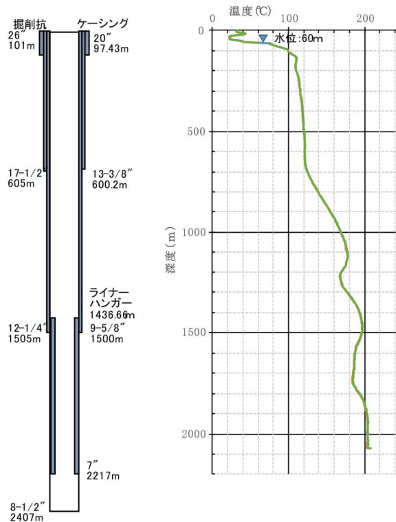
Fig. 7.1.4 (Right) Temperature measurements of F1 geothermal borehole measured by DTS mode. (Left) Casing plan of F1 borehole.
