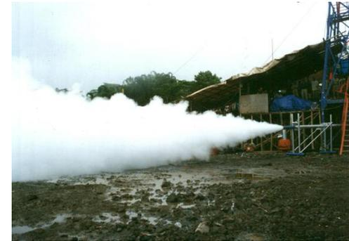
Photograph of 15 tons per hour of steam production of the NEDO MT-2 well. It was only the 162.35 m depth well because of the drilling in the remote island (Sueyoshi et al., 2002).
