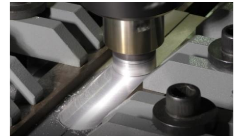
FSW (Friction Stir Welding 摩擦攪拌接合)
