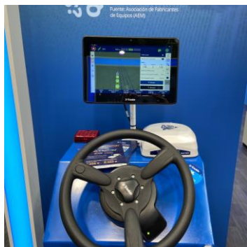
Basic kit consist of steering for ISOBUS, GNSS receiver and monitor
