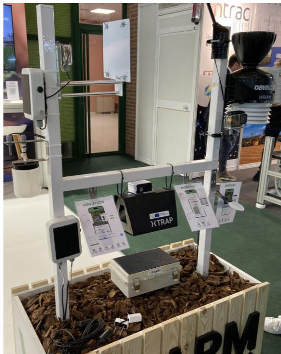
xFarm's weather, soil humidity and pest sensors. Operated through their digital farming software.
