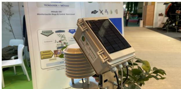
IG4's Weather and soil (humidity, nutrients) sensors
