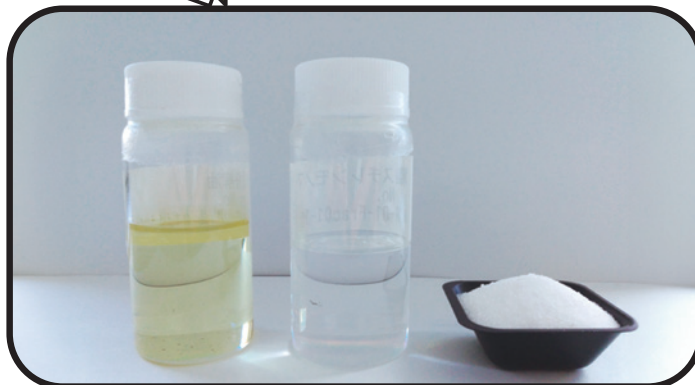
Oil is decomposed from waste polystyrene using microwave technology (left). Styrene monomer is recovered from the decomposed oil (center). The styrene monomer is then re-polymerized and used to produce recycled polystyrene (right).
