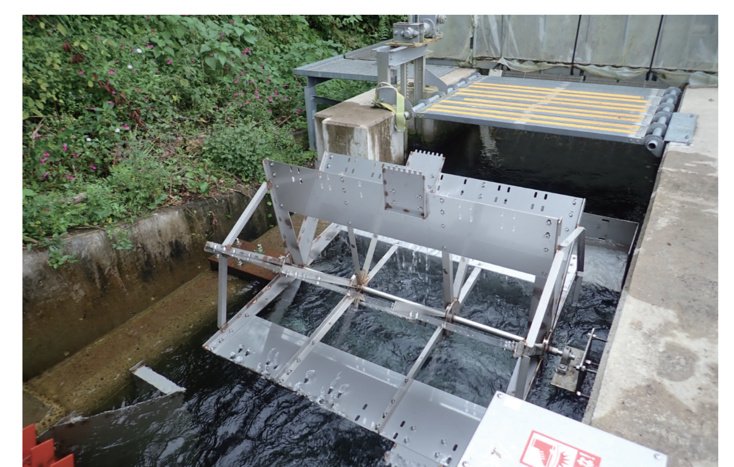
Non-electric garbage remover Source: Aratani Civil Engineering Consultants Co., Ltd.
