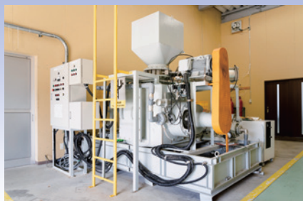
Pulper separator that separates and recovers paper pulp and aluminum mixed with plastic from aluminum waste
