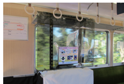
The transparent display was installed on the windows of trains running on a test track owned by Mitsubishi Heavy Industries, Ltd. In this verification, a non-transparent film was hung to verify the case in which a transparent display is used on smoked glass. (Data provided by Sharp Display Technology Corporation)
