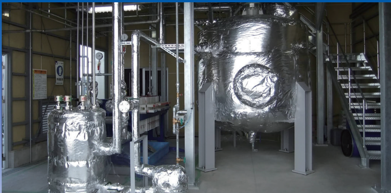
Hydrogen production system that produces hydrogen from extracted aluminum (Data provided by Alhytec Inc.)
