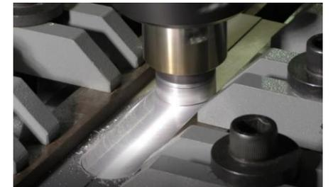
FSW (Friction Stir Welding 摩擦攪拌接合)
