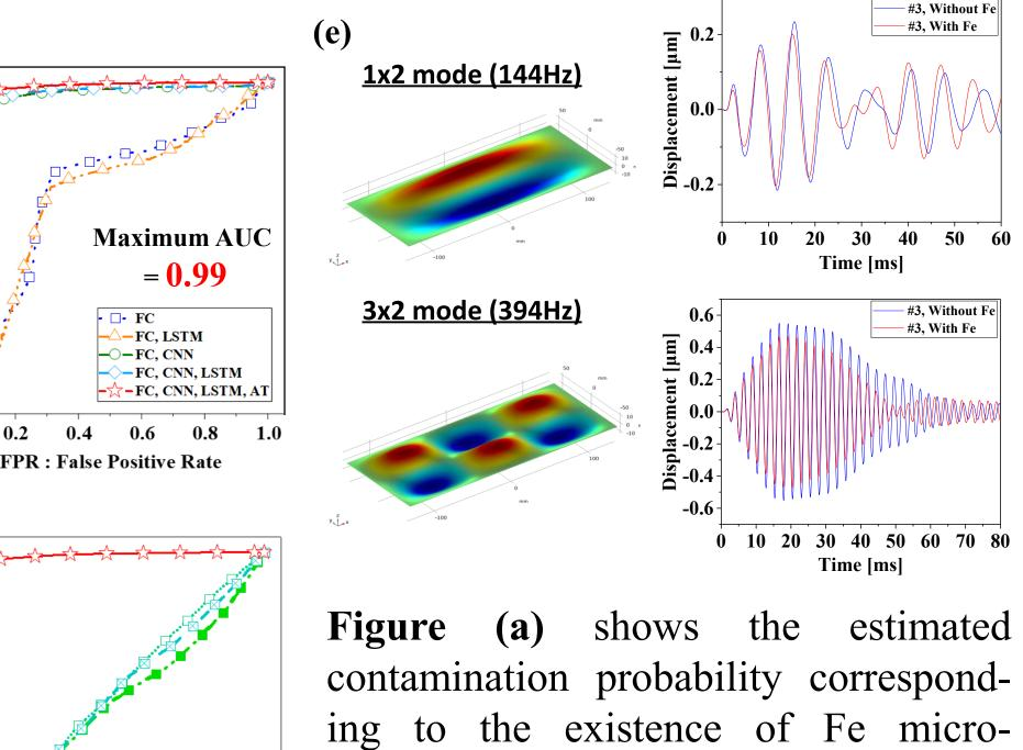
particles buried in MEA. There appears to be more than 90% difference in the contamination probability between presence and absence of Fe micro-particles,
