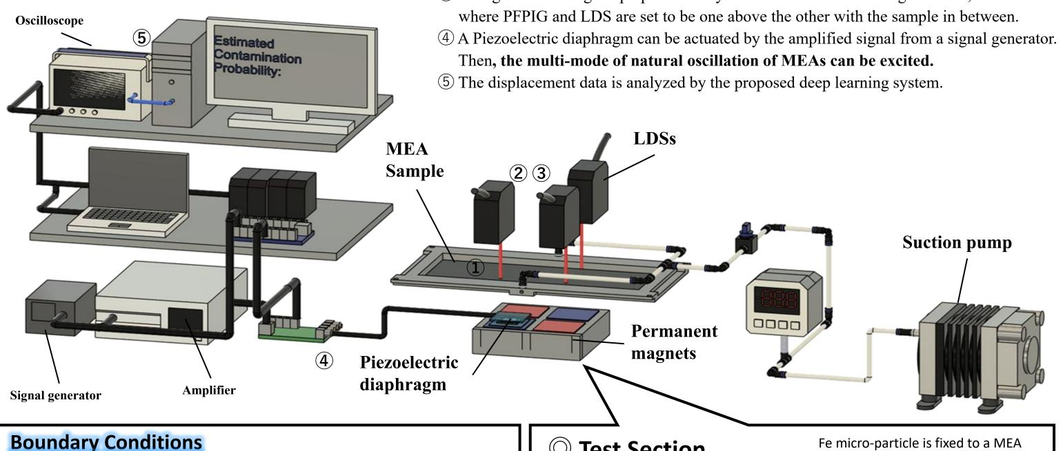
eddy current and magnetic field can generates Lorentz force. When metallic micro-particles are buried into MEA, Lorentz force should be
