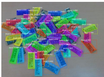
Loose-stacked recognition (irregular shape handling)
