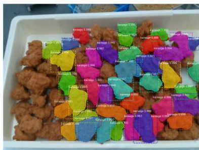
Loose-stacked recognition (irregular shape handling)
