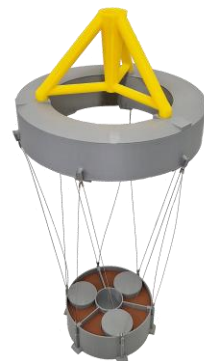
Double-Donut Spar-Type Floating Structure Fundamental Structure of the Double-Donut Spar
