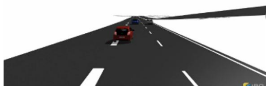
Fig.3-6-8 Simulation-based evaluation of ACC control (Target following distance: 20 m)
