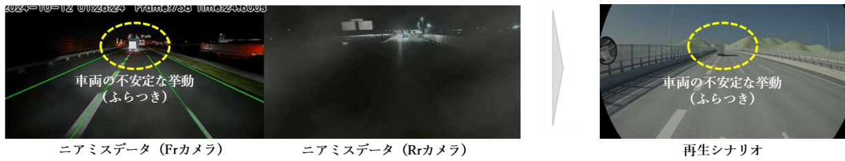
Fig. B-3 Replication of lane departure caused by the wobbling of the ahead vehicle Using DIVP DIVP 活用での前方車両のふらつきによる車線逸脱再現
