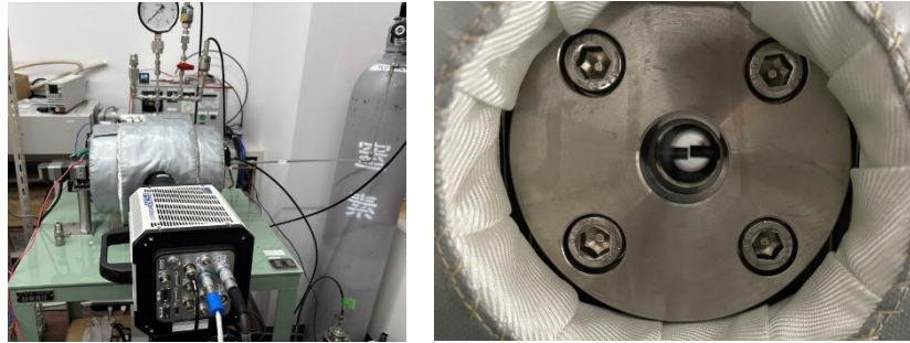
Figure 0-3 Overall view of the electrical-short device and enlarged view of the electrodes
